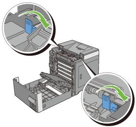
7 Confirm that there are no scraps of paper remaining inside the printer, and then close the belt unit.
